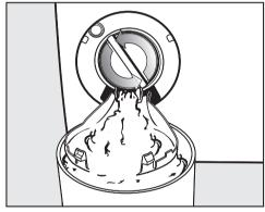
■ Instead, loosen the drain filter enough to allow the water to drain out.
